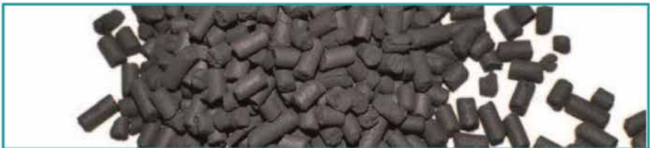
Activated carbon granules
